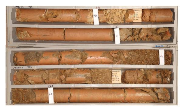
Figure 5:: Photo of a section of drill core from GNBDD022, 60-63m 3m at 3,223ppm TREO, including 1m at 7,956ppm TREO, 1,090ppm Nd and 240ppm Pr from 61m, this interval sits within the larger interval of 8m at 1,854ppm TREO from 57m downhole.
