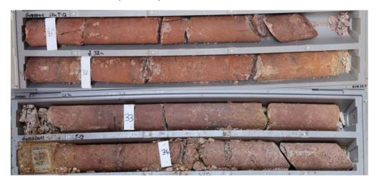
Figure 4: Photo of a section of drill core from GNBDD011, 3m at 3,481ppm TREO from 31m, this interval sits within the larger interval of 27.4m at 1,426ppm TREO from 26m downhole
